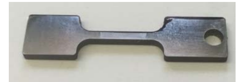
Welded 740H sample - etched
