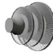
3-stage Single Turbine Hi → Lo 1 meter sCO 2 (300 MWe) (Brayton Cycle)
