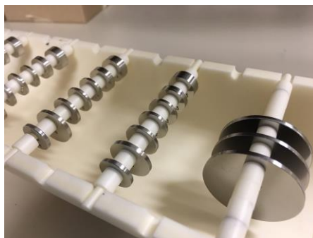
Figure 5. Aluminum oxide sample holder fabricated for the alloy corrosion experiments
