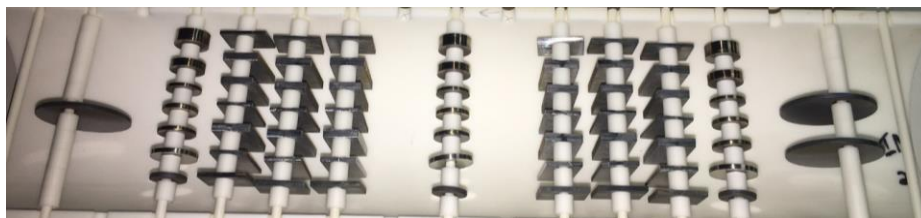
Figure 8. Sample holder showing the inclusion of supplemental metal loss coupons (rectangular)
