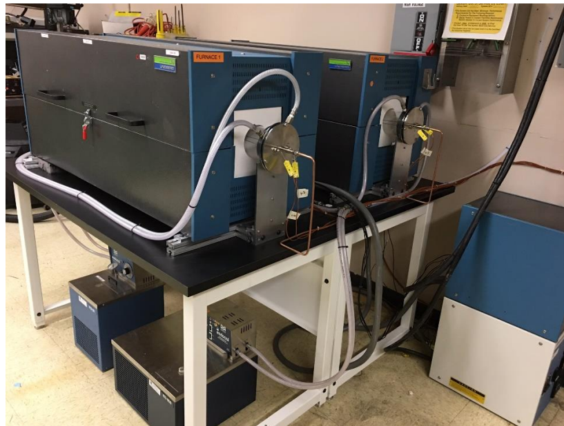
Figure 4. Two large tube furnace setups used for alloy corrosion experiments
