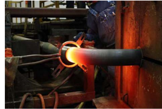
Induction Bending at CB&I
