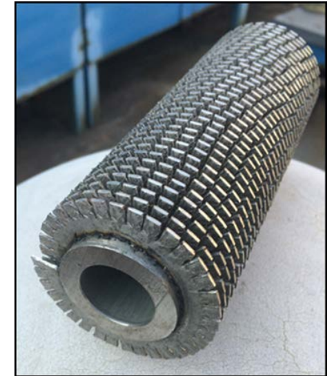
304 Fins resistance welded to 740H, Optimus, Chanute, KA
