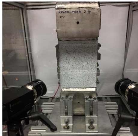
Hydrotest setup with cameras set for 3-D digital image correlation (DIC)
