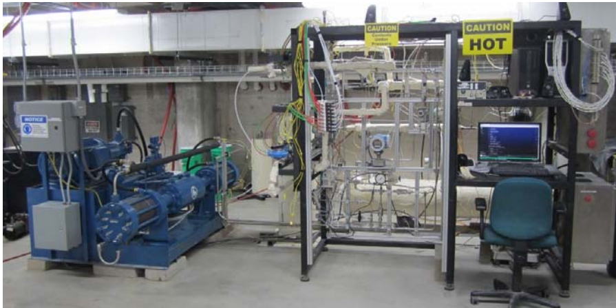
High DP HydroPac supercritical CO 2 loop. Used for heat exchanger, component, and systems testing.
