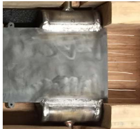
PCHE with capillary tube for temperature sensing fibers
