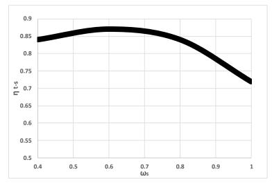
Fig. (7) – Typical total to static efficiency vs. specific speed for radial single stage turbines
