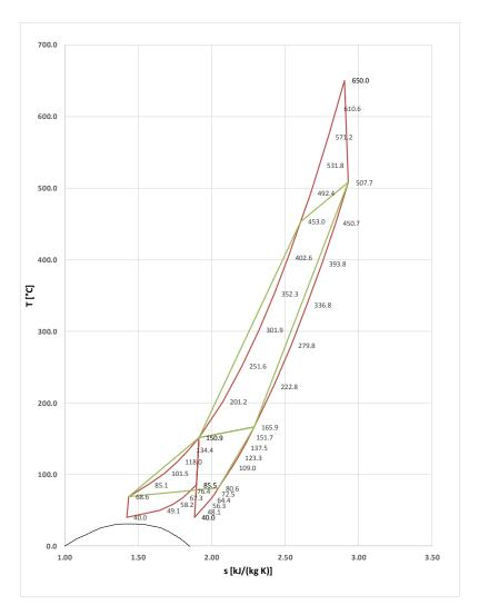
Fig. (1) - Recompressed and intercooled non-condensing cycle - Demo plant
