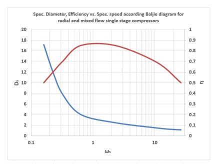
Fig. (6) – Specific diameter vs. specific speed extracted from Balje diagram for radial and mixed flow single stage compressors
