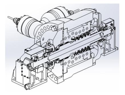
Fig. (5) – Demo plant main turbine sectional view
