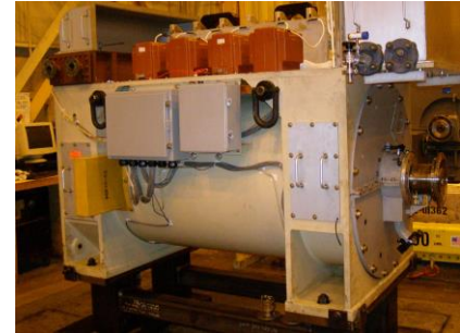
Figure 28. Curtiss-Wright 14 MW 7000 rpm induction generator
