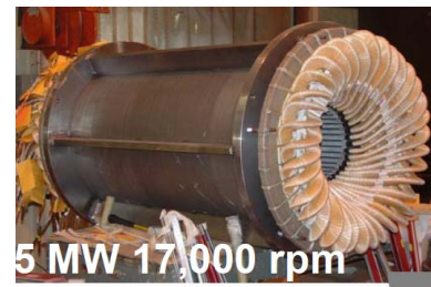
Figure 30. General Electric 5 MW 17,000 rpm PM generator
