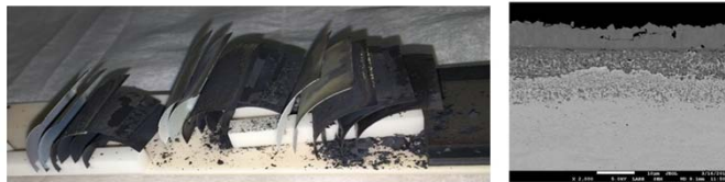
Figure 5: TX1 coating spallation (left) and oxidation (right) for 550°C exposure
