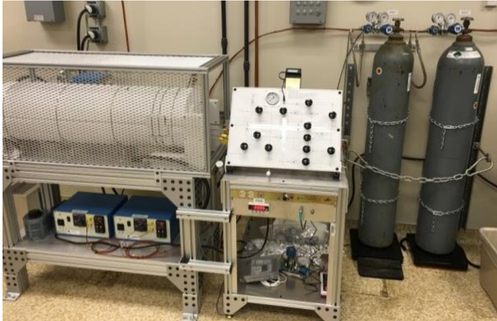
Figure 6. Modified autoclave furnace for gas foil bearing tests at 300psi CO 2
