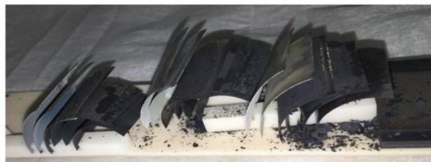
Figure 14. Oxide scale spallation for the TX1 coating exposed at 550°C
