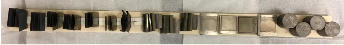
Figure 8. Sample holder loaded up with the full complement of samples for an exposure test
