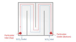
Figure 1: Axial Counter Flow Fluidized Bed
