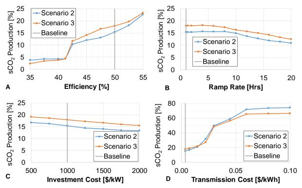
Figure 6. Results of varying the following parameters on the deployment of a distributed sCO<sub>2</sub> power plant: (A) Efficiency, (B) Ramp Rate, (C) Investment Cost, (D) Transmission Cost
