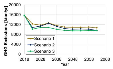
Figure 5. Comparison of baseline scenarios over the model time horizon with respect to: greenhouse gas (GHG) emissions (carbon dioxide)
