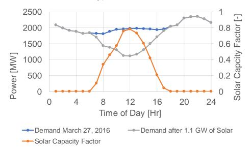
Figure 2. Prediction of "Duck Curve" in Puerto Rico if 1.1 GW of Solar were installed
