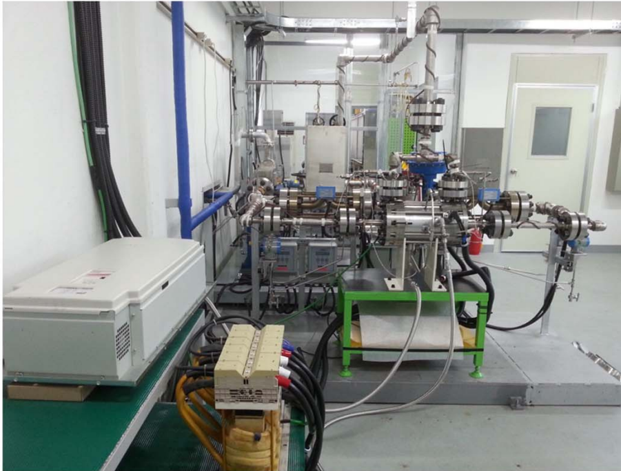
Fig. Compressor Performance Test Loop
