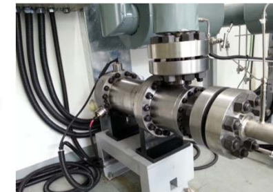
Fig. S-CO 2 turbine and generator
