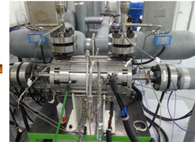
Fig. Double-sided suction S-CO 2 compressor
