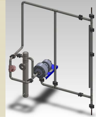
600 °C / 1112 °F - 3600PSI In625 sCO 2 Loop - 160GPM
