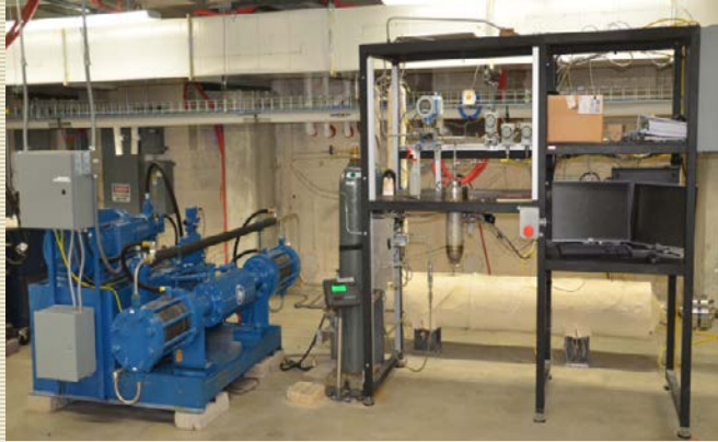
Valve, seal, high speed flow test facility
