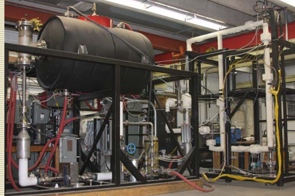
600 °C / 1112 °F - 3600PSI In625 sCO 2 Loop - 160GPM
