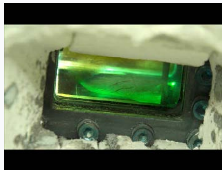
Fig. Potential Na-CO 2 interaction in Printed Circuit Heat Exchanger(PCHE)
