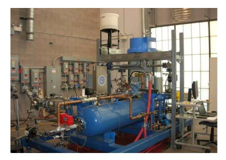
sCO<sub>2</sub> Bearings, Seals and Compressor research platform
