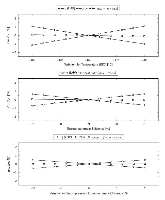
**Figure 4:** Sensitivity analysis for variations in turbine inlet temperature, turbine isentropic efficieny and the recompression turbomachinery efficiency. These diagrams show the cycle efficiency  $\eta$  and the exergy destruction coefficient of the overall cycle  $y_{tot}$  as well as the effect that the exergy destruction of the respective component(s) has on the exergy destruction coefficient of the other components.
