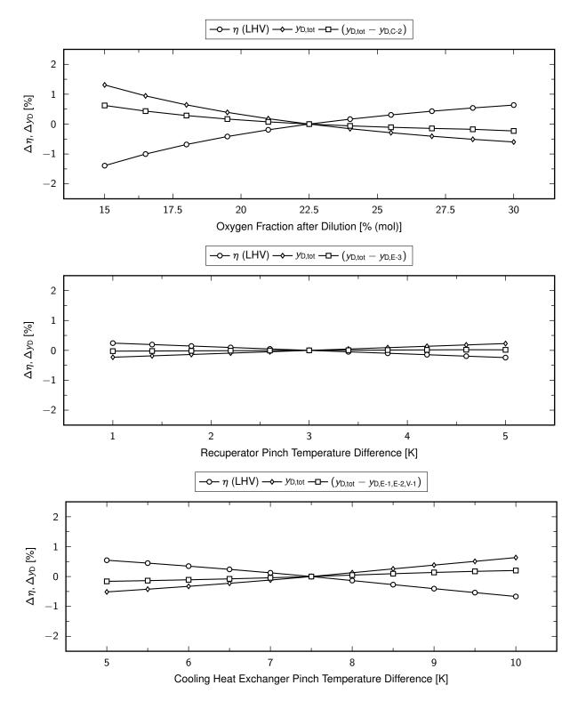
**Figure 5:** Sensitivity analysis for variations in oxygen fraction after dilution and pinch temperature difference in the recuperator and the coolers. These diagrams show the cycle efficiency  $\eta$  and the exergy destruction coefficient of the overall cycle  $y_{tot}$  as well as the effect that the exergy destruction of the respective component(s) has on the exergy destruction coefficient of the other components.
