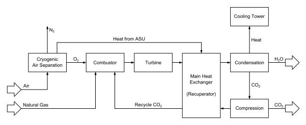
Figure 1: Process diagram of the Allam cycle
