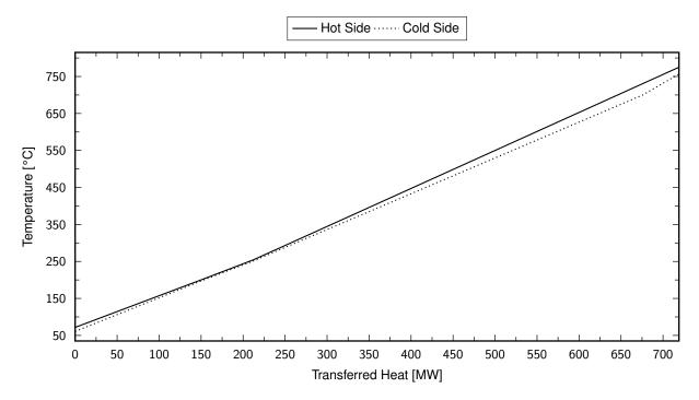
Figure 3: Composite curve of the recuperator
