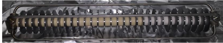
Fig. 2. Photograph of the Inconel 625/Alumina sample holder
