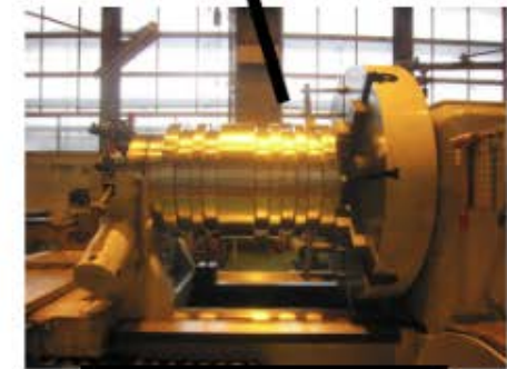
Center Rotor; Ni base Forging
