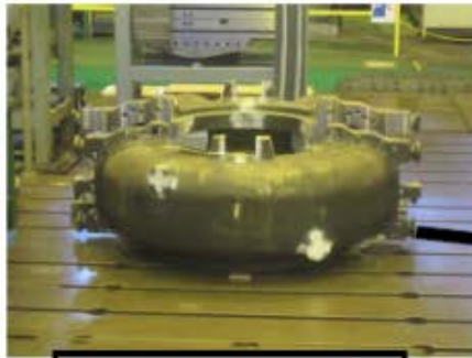
Inner Casing; Ni base casting
