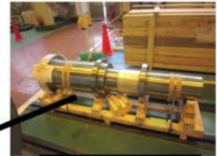
Aft rotor; CrMoV Forging
