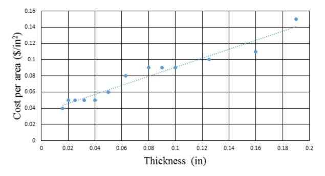
Figure 4. Cost of fin material per unit square area plotted versus sheet thickness.
