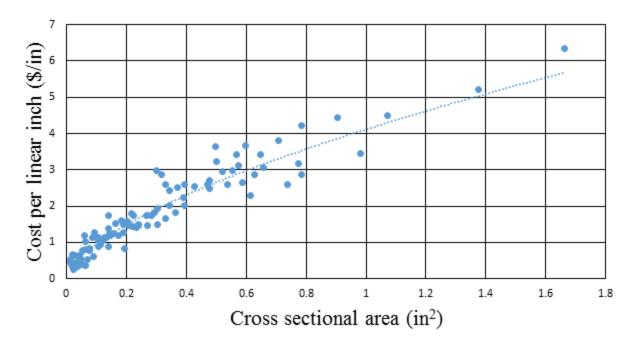
Figure 3. Cost of tubing material per unit length plotted versus cross sectional area.
