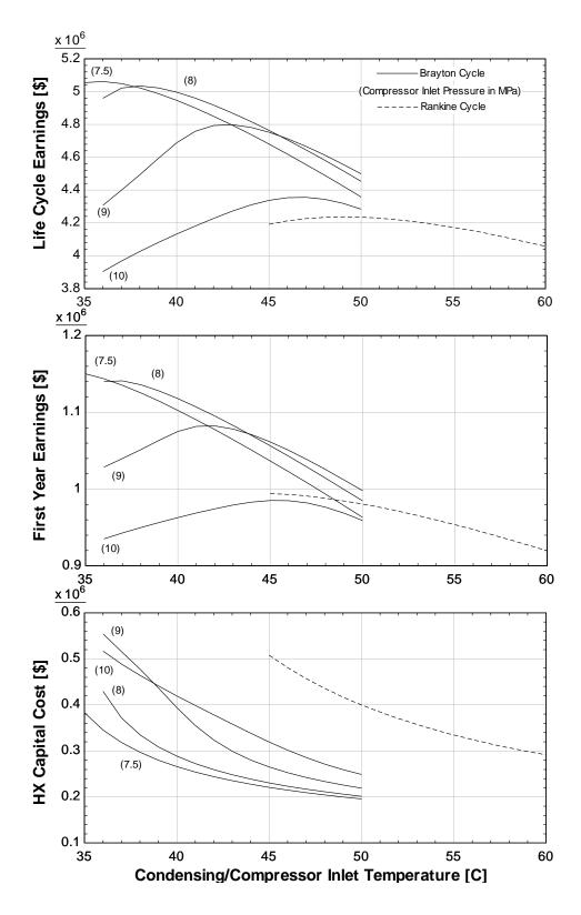
Figure 6. Cost breakdown plotted versus condensing temperature and compressor inlet temperature for different compressor inlet pressures. Compressor inlet pressure in MPa shown in parentheses.
