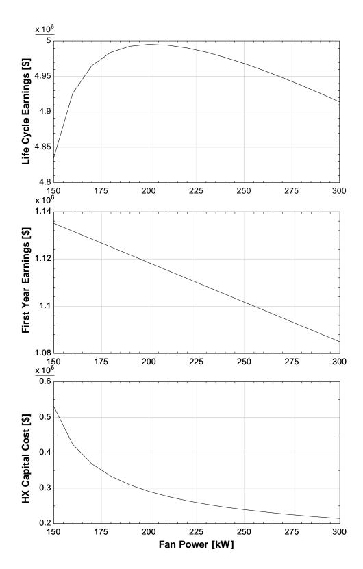
Figure 5. Effect of fan power on the life cycle earnings analysis for the Brayton cycle.
