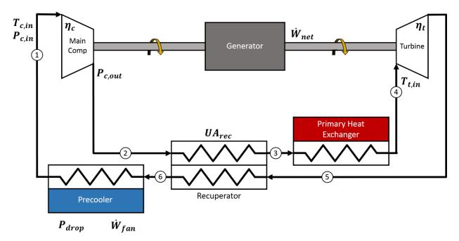
Figure 1. Diagram of the simple Brayton cycle with recuperation. Model inputs shown in bold.
