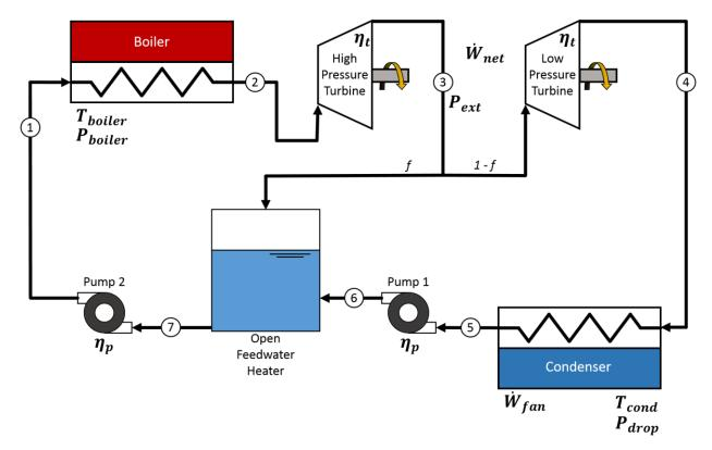
Figure 2. Diagram of the Rankine cycle with open feedwater heater. Model inputs shown in bold.
