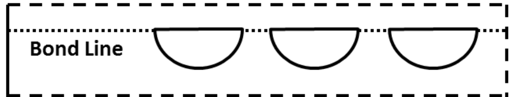
Section of a printed circuit heat exchanger
