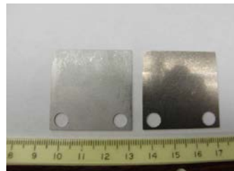
Cold rolled and 1232 °C solution annealed - 550 μm H230 shims
