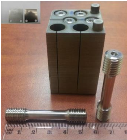
Fig. 2: H230 diffusion bonded stack and tensile testing specimens machined from the stack. The inset shows the H230 sheets before they are bonded.
