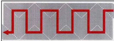
Multipass counter flow example with equal multi passes on both sides.
