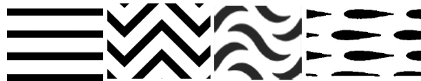
Figure 1. Four PCHE Surfaces: Straight, Zigzag, S-shaped Fin and Airfoil Fin Channels (Left to Right).
