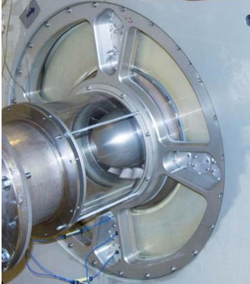
Figure 18. Window placement on test compressor at NTNU wet gas test facility [17]
