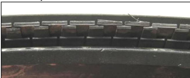
Figure 10: Leaf Tip Burr - Post Wear-in (View from Bottom)
