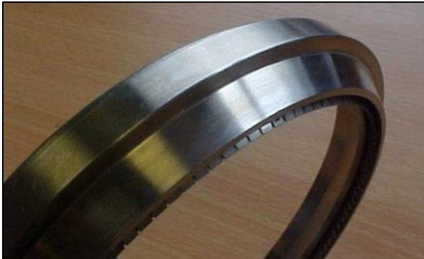
Figure 4: PALS 5.1in (130mm) Diameter Test Seal
