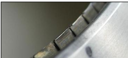
Figure 11: Leaf Tip Burr - Post Wear-in (View from Top)
