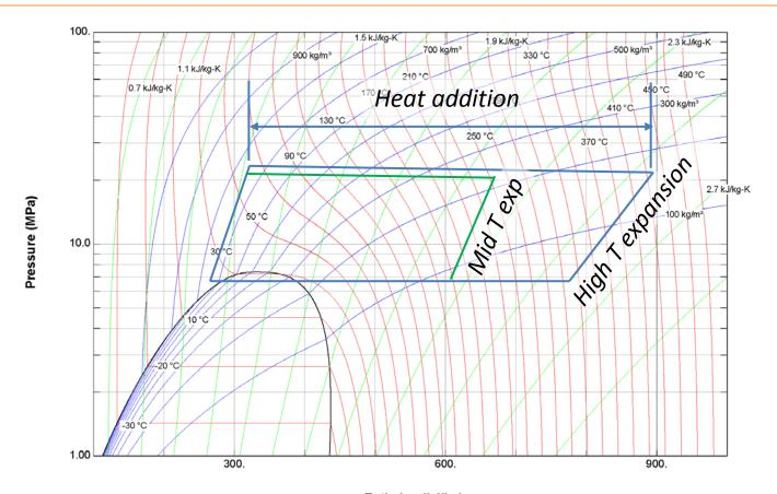
Multiple stages of heat transfer and expansion used to maximize power output for a given heat source  $mc_p\Delta T$
