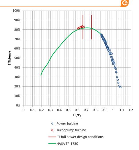
Turbine performance vs NASA TP-1730 curve. Note that TP-1730 curve ends at approximately Ut/C0=0.9.
