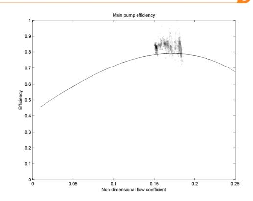
Measured pump efficiency vs flow coefficient. Note that this is a "cloud plot" of the density of approximately 25,000 data points - the gray scale indicates the density of data points that fall within a given x,y coordinate set.
