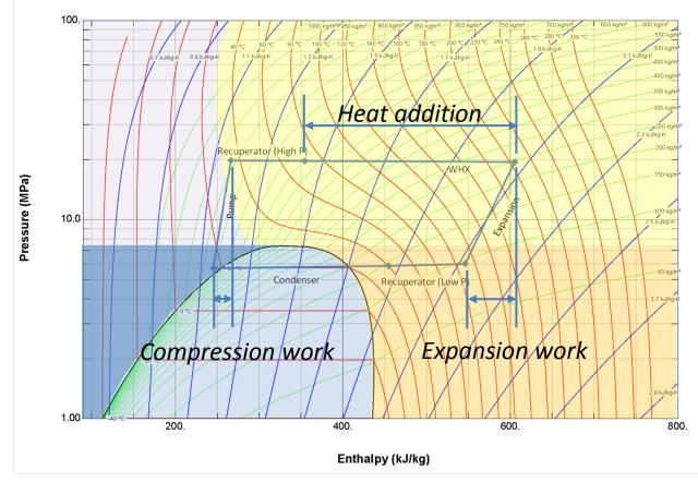
Low pressure ratio cycle => recuperation => can limit  $\Delta T$  of heat addition
