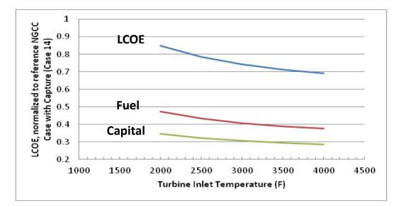
Idealized LCOE predictions – no accounting made for efficiency penalties resulting from approaches incorporated to allow increased turbine inlet temperature
