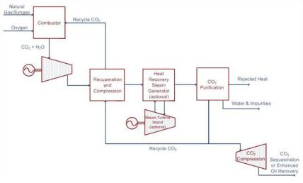
Figure 2: Directly Heated Recuperated Brayton cycle
