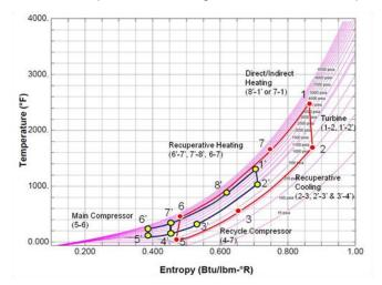
Figure 5: T-S Diagram for Cycle with Constrained Turbine Exit Temperature
