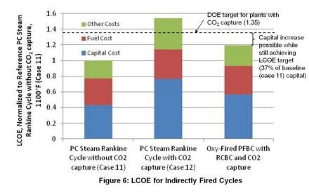
The differences in efficiency, and hence fuel costs, are small between the three cases, but the capital cost for the carbon capture equipment is large. significantly so for the postcombustion capture case. An RCBC plant is predicted to increase LCOE over a PC plant without CO<sub>2</sub> capture by 18%, which only is significantly less than the current DOE targets of 35%. It is also predicted that capital costs could increase
