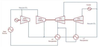
Figure 1: Indirectly Heated Recompression Brayton Cycle
