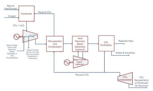
Figure 4: Directly Heated Cycle with Turbine Blade Cooling
