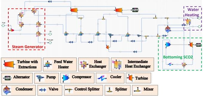
Figure 3. Combined Complex Steam-SCO2 CHP Plant
