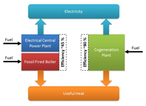
Figure 1. CHP Process Flow Diagram.
