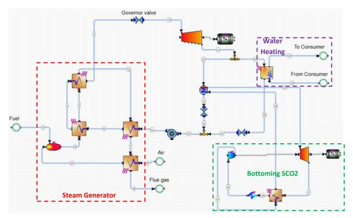
Figure 4. Combined Simple Steam-SCO2 CHP Plant
