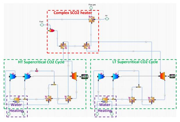
Figure 5.Cascaded Supercritical CO2 CHP Plant
