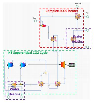
Figure 6. Single Supercritical CO2 CHP Plant
