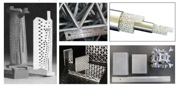
Figure 8. From left to right: internally-cooled turbine airfoil with its intricate casting core, examples of lattice block materials, and both stochastic and ordered metal foams. All of these parts are cast using processes similar to those suggested for CMHEs.
