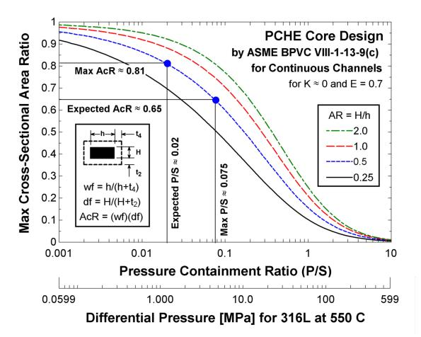
Figure 1. A plot of PCHE core cross-sectional area (or porosity) versus pressure containment ratio or the design differential pressure of a 316L unit for a design metal temperature of 550 °C.
