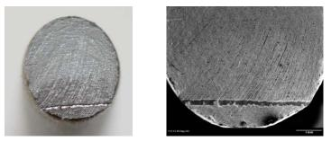
Figure 4. Photograph and SEM image of one side of the failure surface of sample A. The trench shown is likely the result of a foreign object inclusion leading to premature failure.
