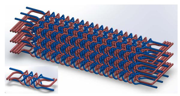
Figure 6. A counter-rotating double-helical geometry proposed for use as a cast metal recuperator between two similar fluids. Red channels depict the "hot" flow side while blue depict the "cold" flow side. Channels from the same side interconnect throughout the body of the unit to themselves and intertwine with channels from the other flow side. Geometric parameters can be optimized to the particular flows involved.
