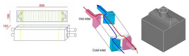
Figure 2. Configuration of the Heatric PCHE tested by Pra et al. (Pra et al., 2008) with V-style headers on the left, as compared with the petal-style header (ALPEMA, 2010).
